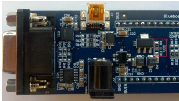
Fig 12. Solder jumper for VCC power supply configuration
