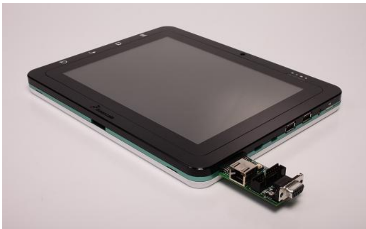
Figure 1-1. MCIMX53SMD Board with a Debug Card and a Display
