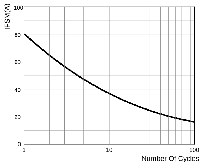
FIG 2: MAXIMUM NON-REPETITIVE FORWARD SURGE CURRENT
