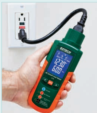
Tests 3-wire standard and GFCI receptacles
