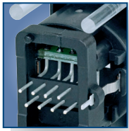
Vertical PCB with lightpipes
