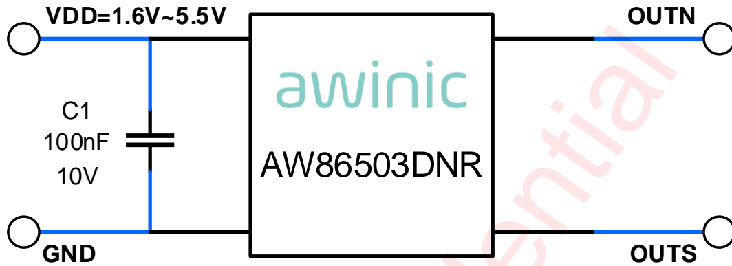
Figure 6 The Application Circuit of AW86503DNR
