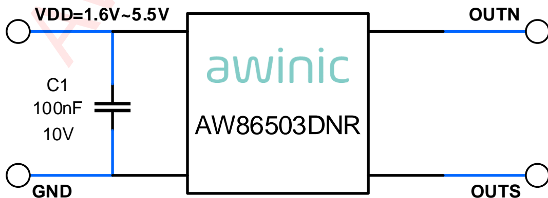
Figure 1 Typical Application Circuit of AW86503DNR
