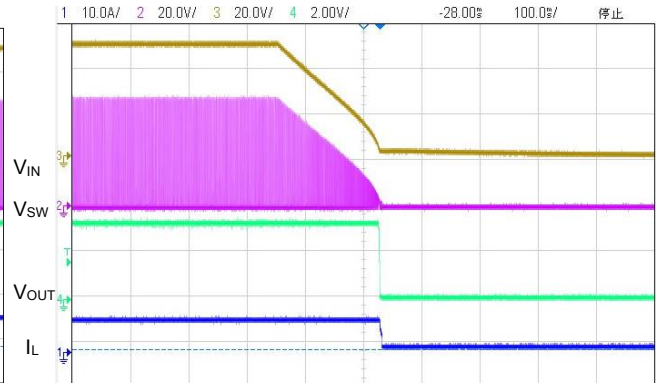
(20) Power Ramp Down ( V_{IN}=50.0V, V_{OUT}=3.3V, I_{OUT}=0.6A )
