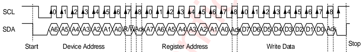
Figure 12 I 2 C Write Byte Cycle
