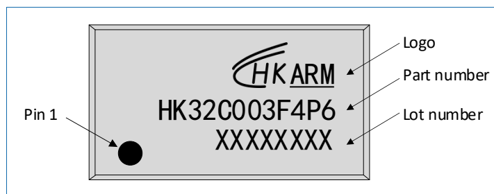
Figure 7-9 TSSOP20 HK32C003F4P6 marking example
