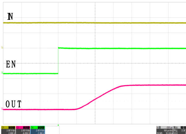
C1: 2.00V/div C2: 2.00V/div t=160µs/div C4: 2.00V/div VIN=3.3V, CIN=1µF, COUT=1µF, Rload=5Ω
