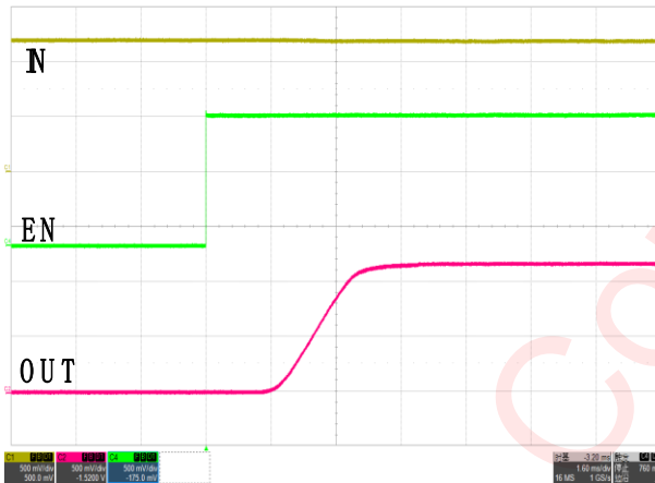
C1: 0.5V/div C2: 0.5V/div t=1.6ms/div C4: 0.5V/div VIN=1.2V, CIN=1µF, COUT=1µF, Rload=5Ω
