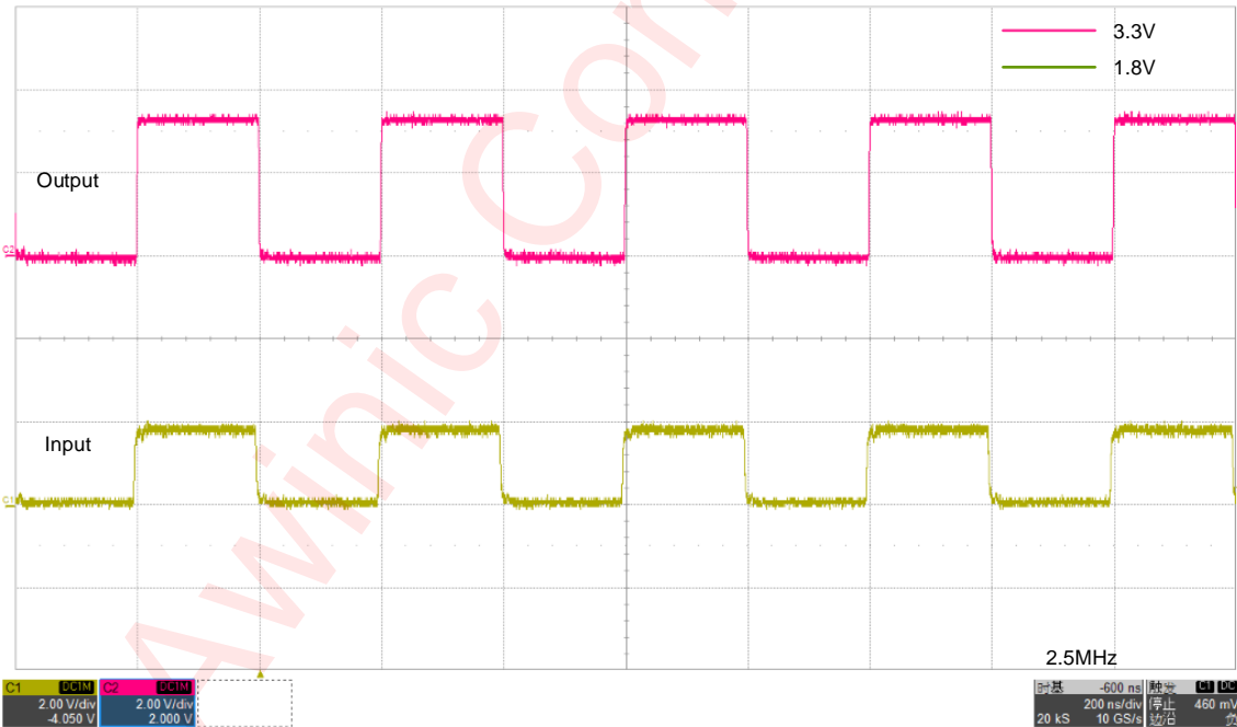
2.5-MHz 1.8V-3.3V Signal Level-Translation @ C_L=30p
