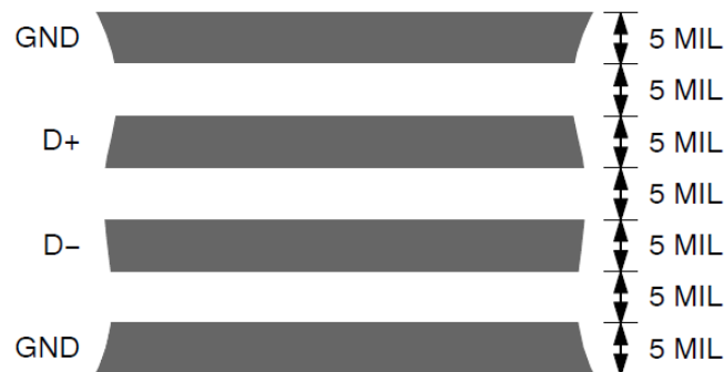
Figure 23. Typical Arrangement of Signal Tracks
