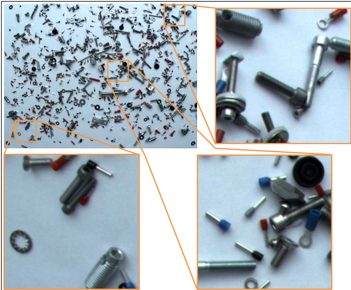
Figure 7: acA2500-14gc, f/2.8 , 0.5 m Working Distance, Full 5 Megapixel Image and Selected Magnified Sections
