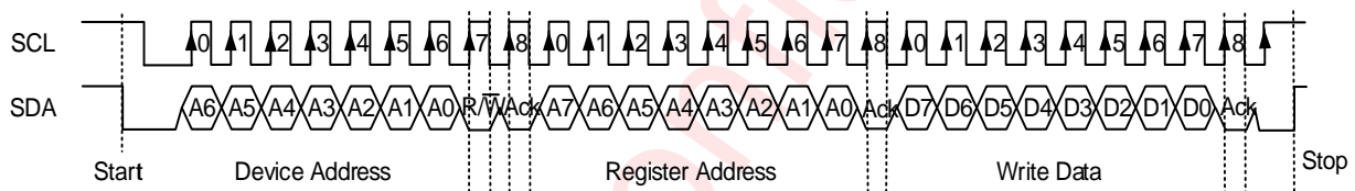
Figure 12 I 2 C Write Byte Cycle
