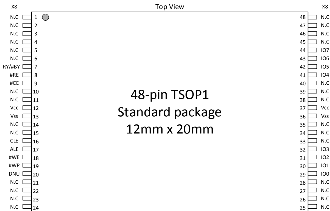
Figure 3-1 Pin Assignment 48-Pin TSOP1 (Package code S)
