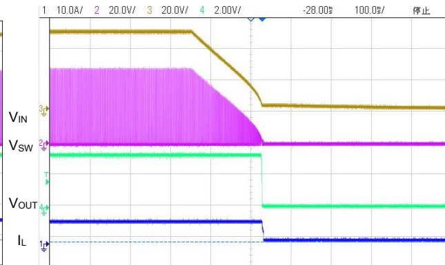
(20) Power Ramp Down ( V_{IN}=50.0V, V_{OUT}=3.3V, I_{OUT}=0.6A )
