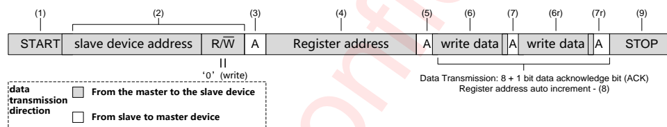
Figure 27 Writing process (data transmission direction remains the same)
