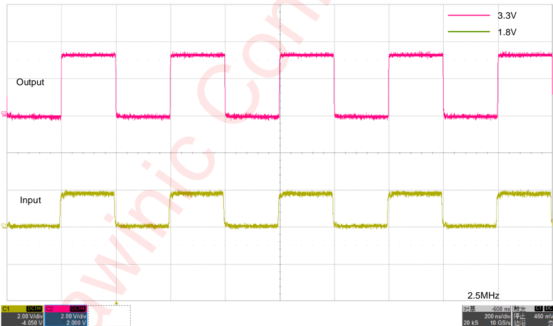
2.5-MHz 1.8V-3.3V Signal Level-Translation @ C_L=30p
