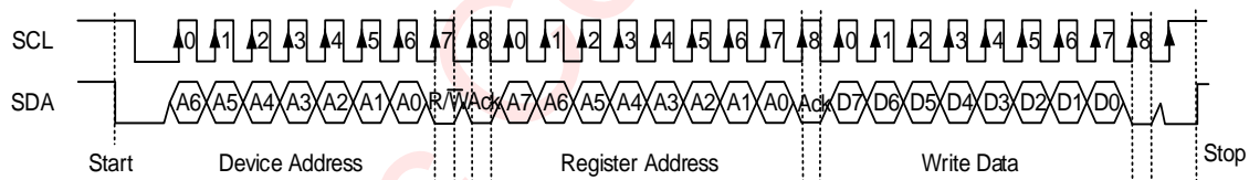
Fig 35 I 2 C Write Timing
