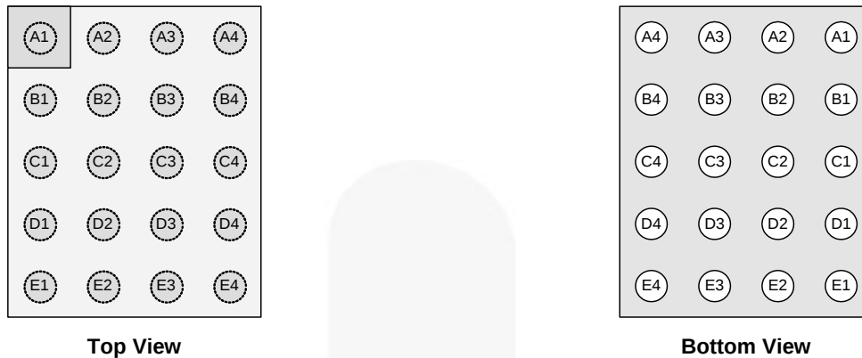
Figure 4. WLCSP-20 Pin Assignments
