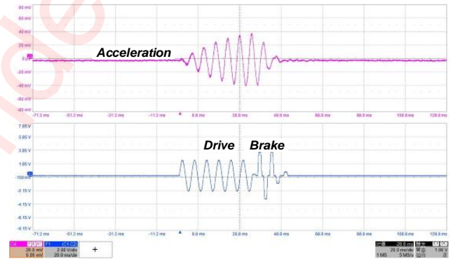
Figure 12 LRA with Automatic Braking
