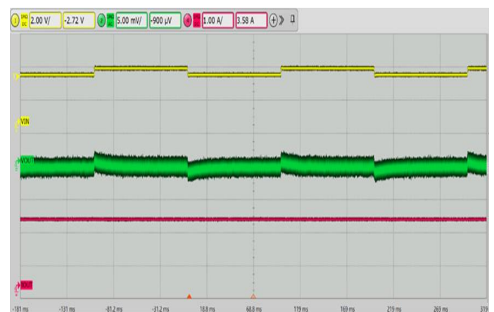
Line transient, V_{IN}=2.7V \sim 3.3V , V_{OUT}=0.6V , I_O=2A
