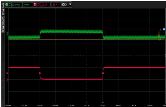
Load transient, V_{IN}=2.7V , V_{OUT}=0.6V (with droop), I_O=0A\sim 1A
