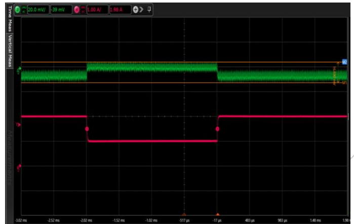
Load transient, V_{IN}=2.7V , V_{OUT}=0.6V (with droop), I_O=1A\sim 2A
