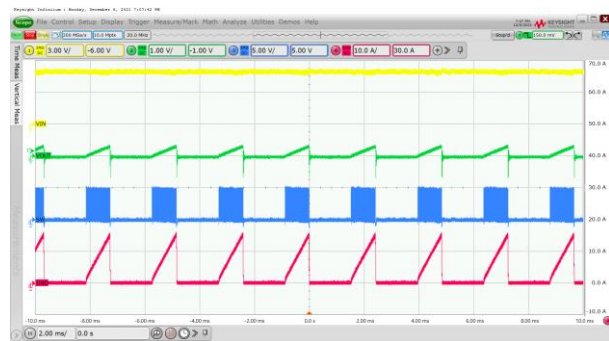
Hiccup With Output short, V_{IN}=5V, V_{OUT}=1.0V , Steady
