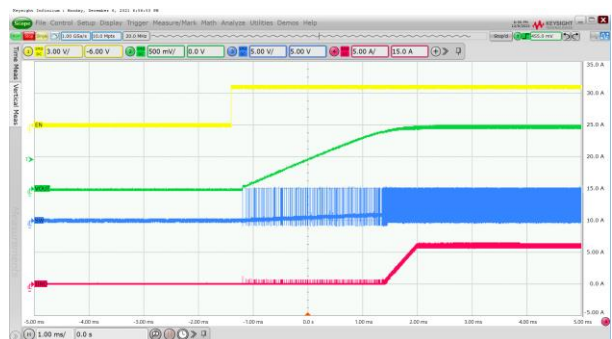
Enable on, V_{OUT}=1.0V, I_{OUT}=6A
