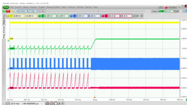
Hiccup With Output short, V_{IN}=5V, V_{OUT}=1.0V , Recovery
