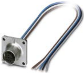
Sensor/Actuator flush-type socket, 5-pos., M12, A-coded, front/square flange mounting, with 0.5 m TPE litz wire, 5 x 0.34 mm²
