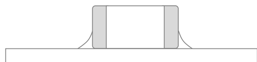
Not enough solder Weak holding force may cause bad connections or detaching of the capacitor
