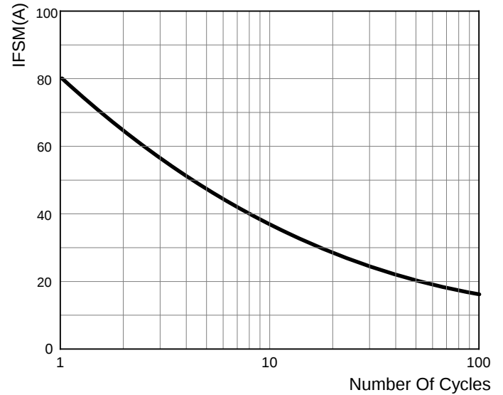
FIG 2: MAXIMUM NON-REPETITIVE FORWARD SURGE CURRENT
