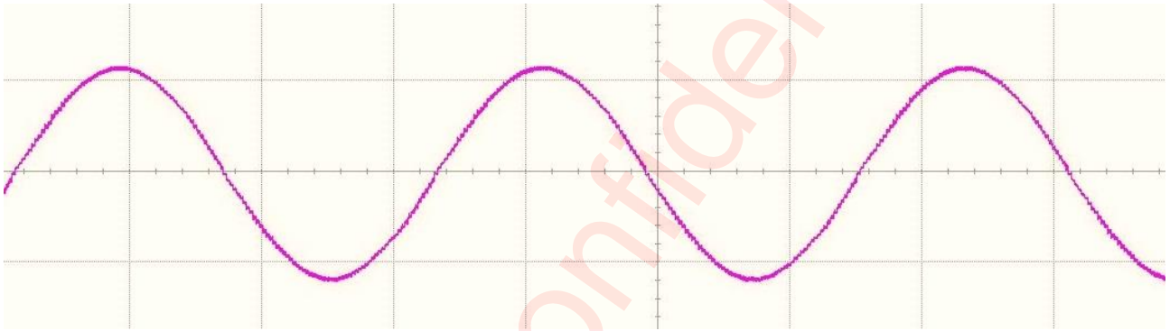
Figure 9 Microstepping Waveform, Phase A, Adaptive Decay
