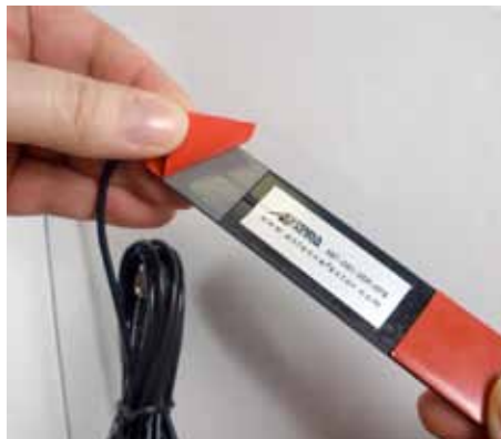
Figure 18. Adhesive Mount Antenna – Step 2. Peel Protection from Adhesive Strip
