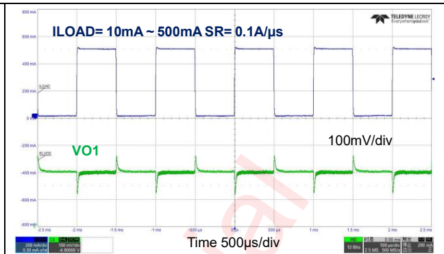
Figure 22. VO1 load transient (10~500mA/SR=0.1A/μs)
