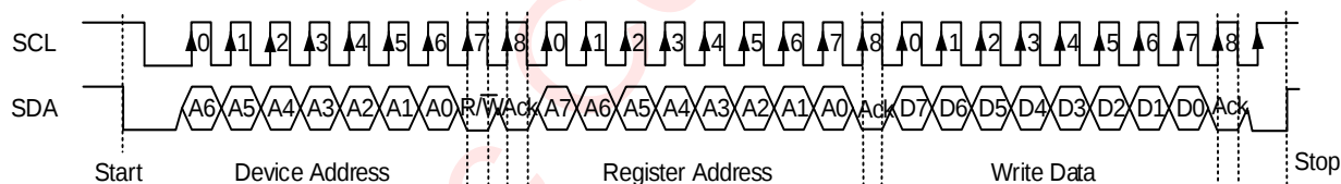
Figure 15 I 2 C Write Byte Cycle
