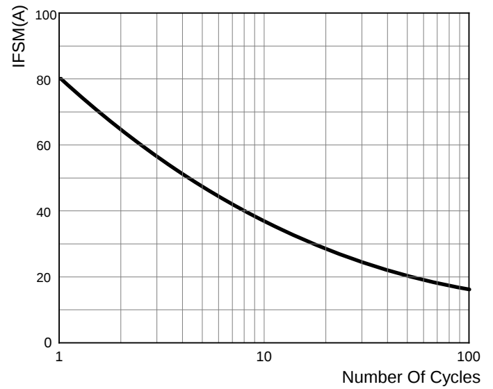
FIG.2: MAXIMUM NON-REPETITIVE FORWARD SURGE CURRENT
