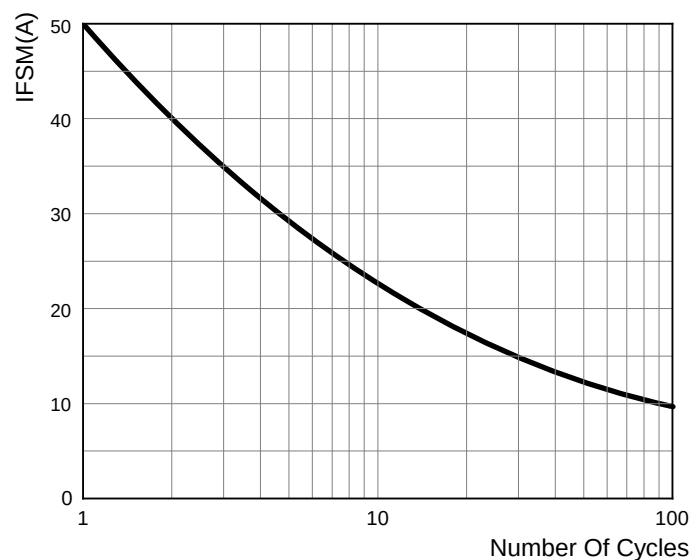
FIG 2: MAXIMUM NON-REPETITIVE FORWARD SURGE CURRENT
