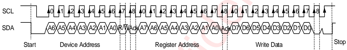
Figure 8 I 2 C Write Byte Cycle
