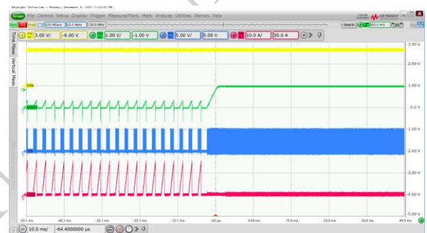
Hiccup with output short, V_{IN}=5V , V_{OUT}=1.0V , Recovery
