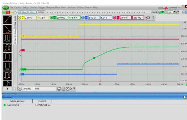
Enable on, V_{OUT}=0.6V , I_{OUT}=0A
