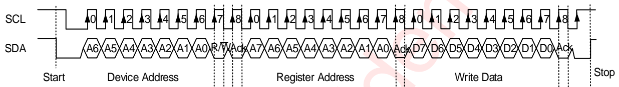
Figure 13 I 2 C Write Byte Cycle
